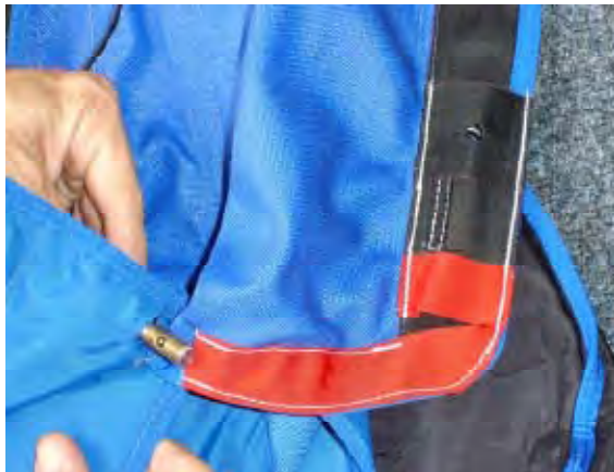
5.1 Thread Cutter thru slit in Panel #1
