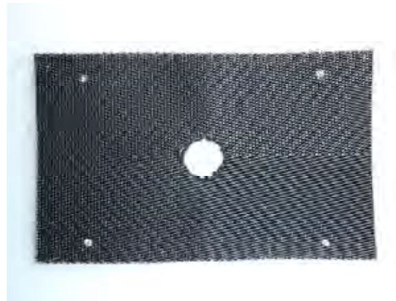
2.4 Cut TYPE 12 Webbing as per Template
