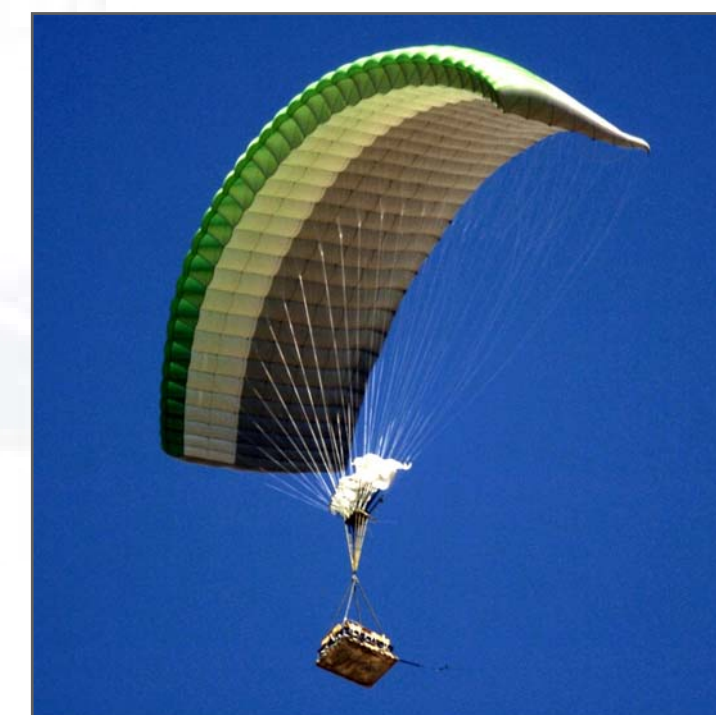
The GPS Guided Joint Precision Aerial Delivery System (JPADS) is critical to reducing casualties to military support units in combat theaters as well as providing humanitarian relief.
