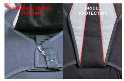
Figure 51. Bridle Routing Check
