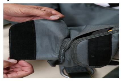
Figure 10. Check the Condition of the Velcro
