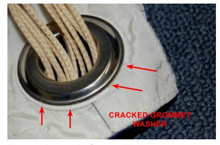
Figure 38. Inspect the Grommet Washer
