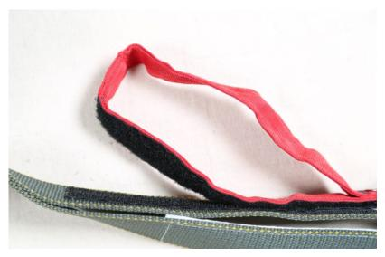
Figure 31. Inspect Velcro Condition
