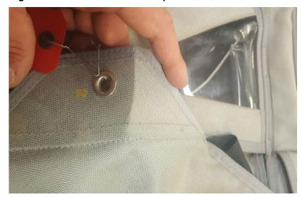
Figure 6. Plastic Stiffener Supporting the Grommet
