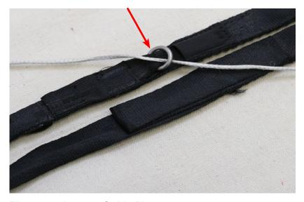
Figure 25. Inspect Guide Rings
