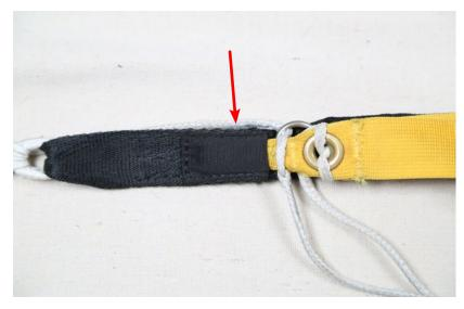
Figure 28. Inspect Toggle Tip Keeper
