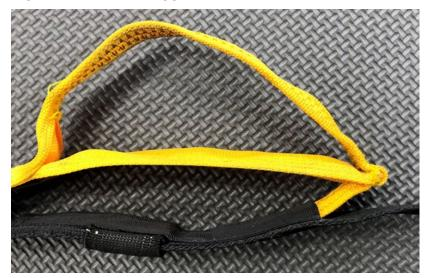
Figure 29. Inspect Tuck Tab Keeper
