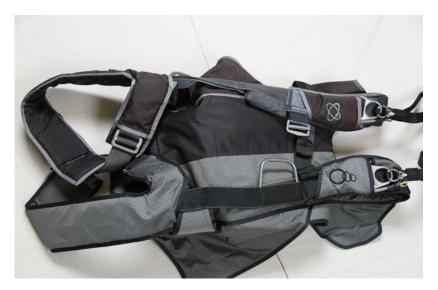
Figure 11. Inspect Harness Webbing for Damage
