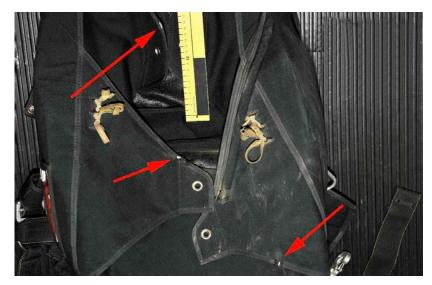
Figure 5. Fabric Abrasion & Exposed Plastic Stiffeners
