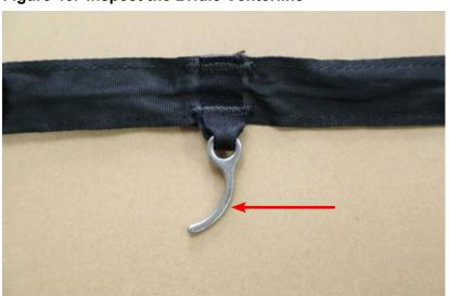
Figure 47. Inspect the Container Closing Pin
