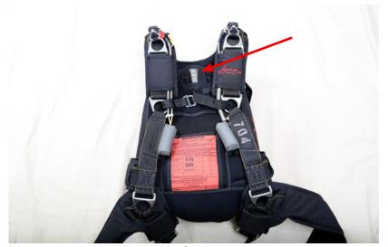
Figure 59. AAD - Properly Calibrated
