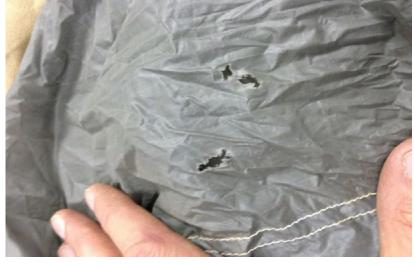
Figure 17. Fabric Inspection – Damage Identified
