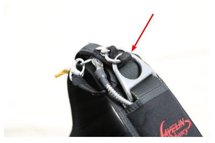
Figure 55. 3-Ring Assembly Check
