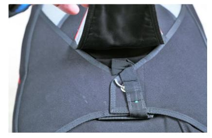
Figure 50. Main Pin and Bridle Check
