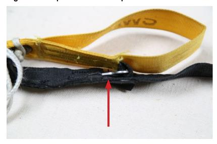
Figure 30. Check Toggle Retention is Secure
