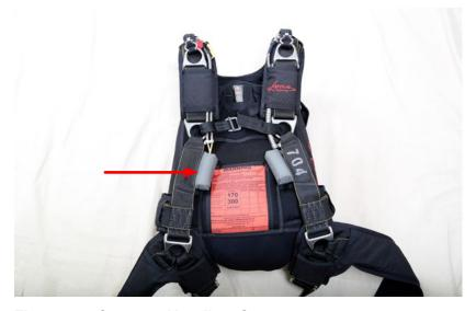
Figure 57. Cutaway Handle - Secure
