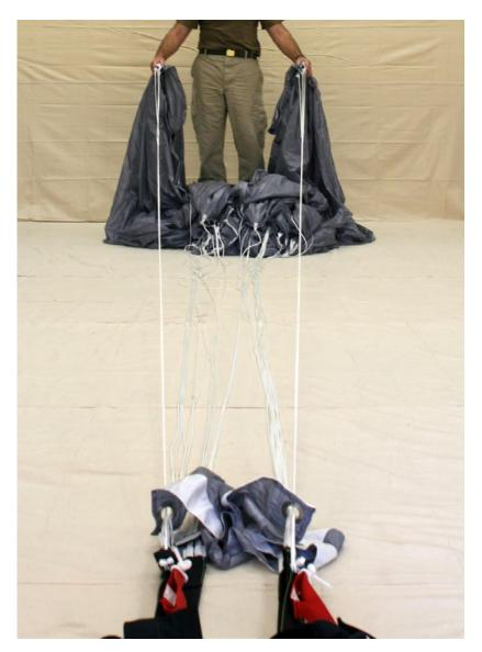
Figure 24. Control Line Check
