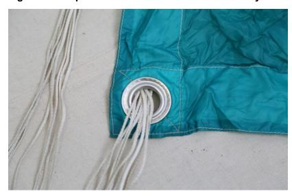
Figure 36. Inspect All Slider Grommets for Damage
