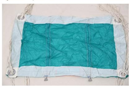
Figure 39. Inspect Fabric and Support Tapes/Webbing
