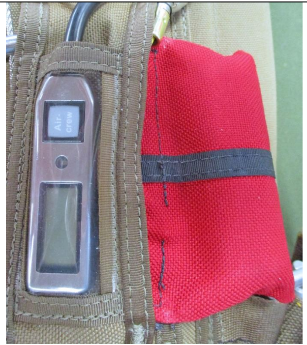
Cable installed – A blank Control Unit means Proper Functionality. If "0" continues to show the unit is defective.
