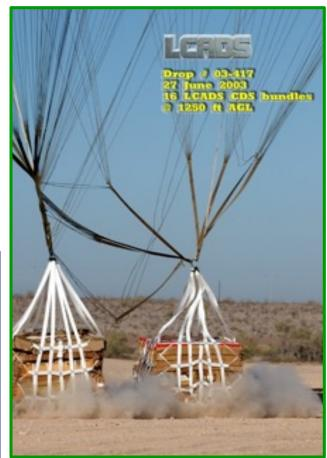
Low Cost Aerial Delivery System (LCADS) High Velocity Parachute
