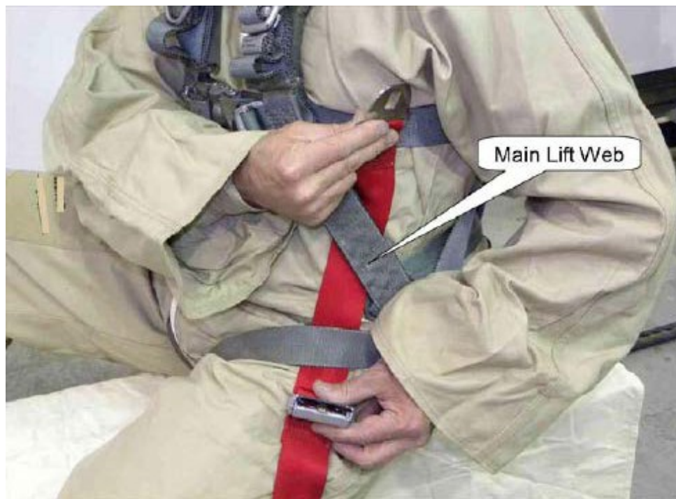
FIGURE 5. PASS TETHER LOOP UNDER MAIN LIFT WEB
