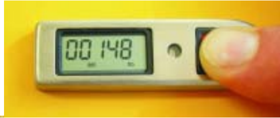
Figure 2a: The CYPRES 2 Control Unit consists of a 5 digit LCD display, a LED and a push-button (Ser.Numb. in display in this case).
