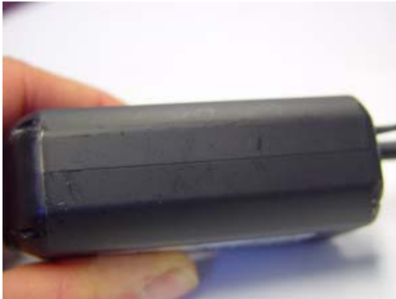
Fig. 13: Minor scratches after 10 drops from 1 meter height and another 10 drops from 2 meters height.
