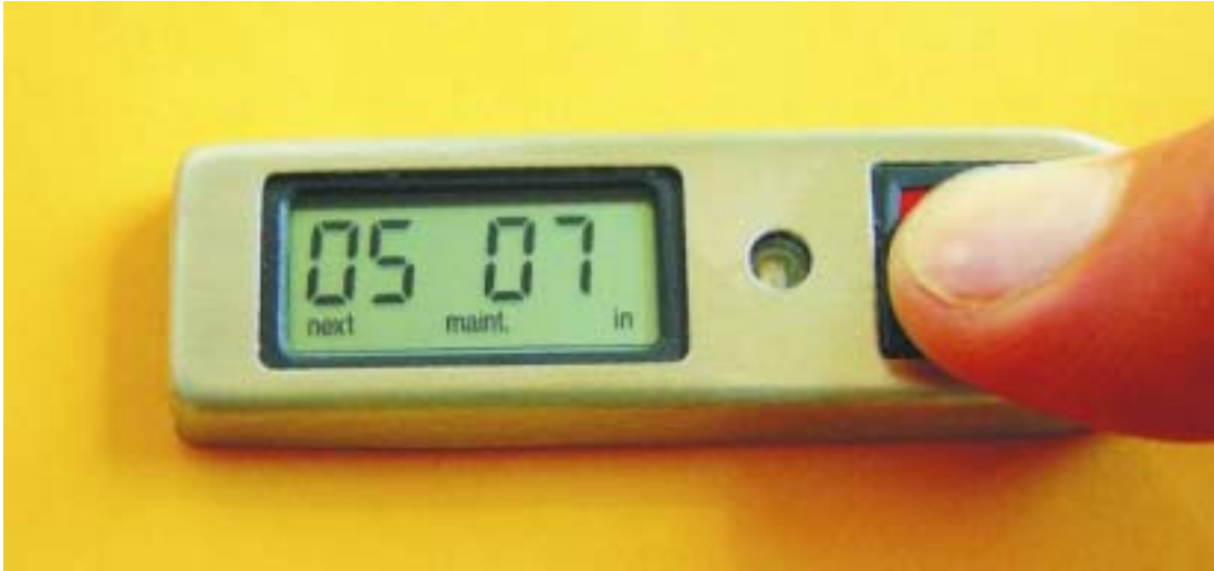
Fig. 8: Example of “Next Maintenance in” indication in the CYPRES 2 display.
