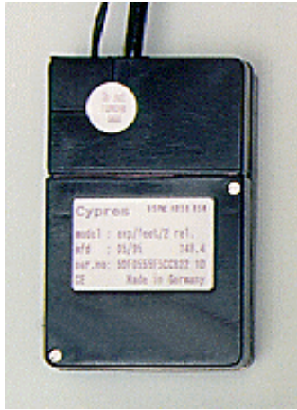
Figure 1: The CYPRES Processing Unit containing the battery, the pressure-measurement system and the processing electronics.
