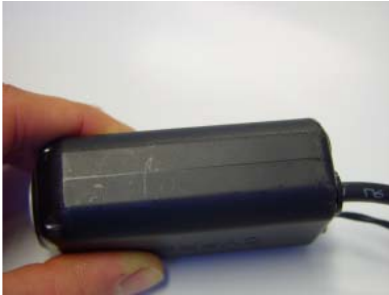
Fig. 14: Minor scratches after 10 drops from 1 meter height and another 10 drops from 2 meters height.
