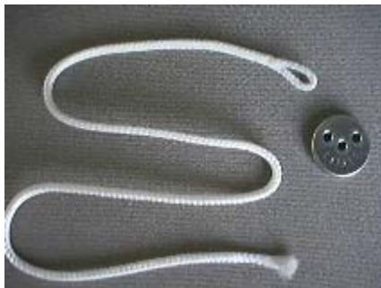
Figure 5: The CYPRES closing-loop and "Smilie" washer.
